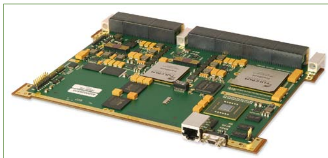
Figure 2 | GE's NETernity GBX460 data plane switch module supports HPEC cluster architectures.
