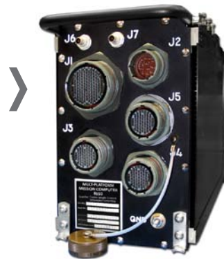
Figure 1 | The ability to integrate high-performance computer power in a small, lightweight mission computer enables the Pilatus PC-21 to perform sophisticated radar system emulation.
